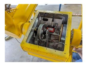
Figure 72 – PTO assembly schematic (left), and photo (right).
